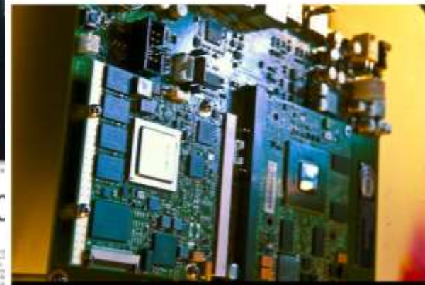
A Tegra 2 system with a GPU processor. Is this the future of supercomputing? Photo: Barcelona Supercomputing Center
